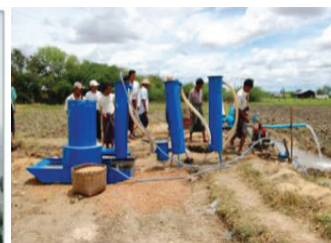
A rice husk gasifier was locally used to power a water pump in Meik-hti-lar Township, Mandalay.
